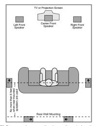
B) Rear speaker mounting is an alternate location for 5.1 systems. It is required for 7.1 operation.
